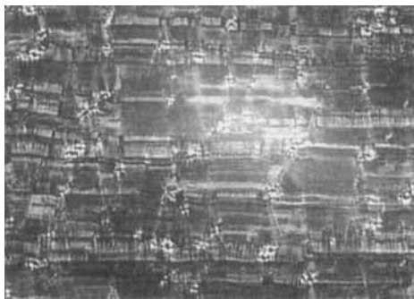
FIGURE 5 Microphotograph illustrating the coexistence of ferroelectric and antiferroelectric states. Vertical edge of the photograph corresponds to 370\text{ }\mu\text{m} . The sample was held for 7 days at 115^\circ\text{C} . See Color Plate XXI at the back of this issue.
